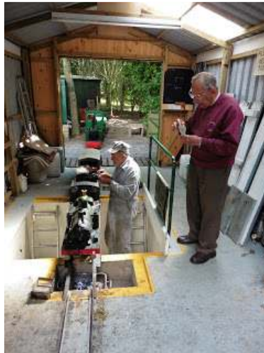
Bob replacing the sight glass in the loco shed pit with Brian R helping
